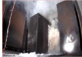
Smoke accumulation at second smoke detector activation [TR + 00:00:55]
