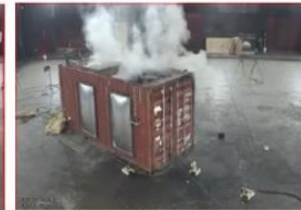
Continued thermal runaway propagation [TR + 00:46:26]
