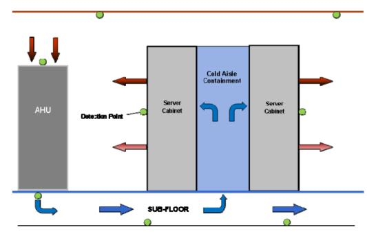
Image: Xtralis Whitepaper – Telecommunications and Data Processing Facilities Design Guide
